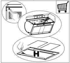
Activated charcoal filter W These filters are not washable and cannot be regenerated, and must be replaced approximately every 4 months of operation, or more frequently with heavy usage.
