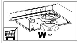
Grease filters ZThe filters must be cleaned every 2 months of operation, or more frequently for particularly heavy usage, and can be washed in a dishwasher.
